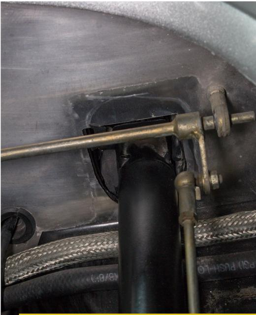
In order the remove the column you will have to remove the firewall plate to allow access to the column. Gently apply pressure to loosen the plate and remove it.
