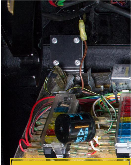
Unscrew the fusebox panel to access the two hinges mounting it at the back of the box. Remove the hinges and combine them with the provided extension plates. Once the plates are assembled reattach them to the fuse panel. Leave the fusebox open as you will need access to the area under the dash. \*Kit car mounting hardware may vary from vehicle to vehicle.
