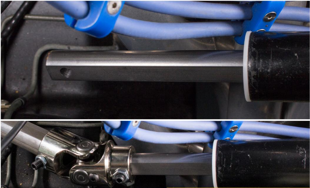
Attach the U-joint to the 3/4"DD shaft coming out of the steering column. Be sure that the set screw fits into the hole predrilled in the 3/4"DD shaft.
