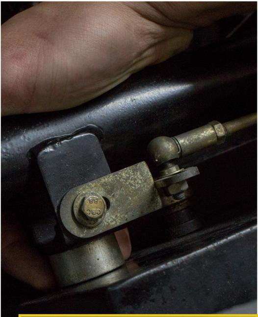
There are two bolts holding the column in place that will need to be removed in order to replace the column. **Do not throw away these bolts** as they will be reused to attach the replacement column. The first is located under the dash above the column and the second is in the engine bay.
