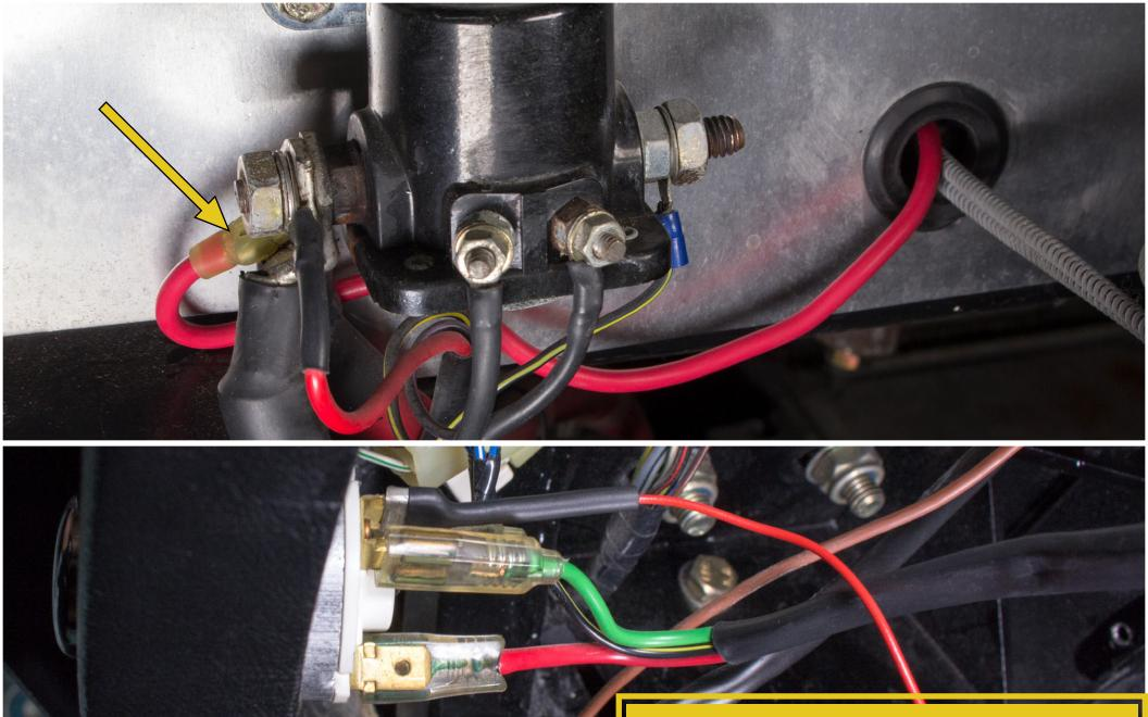
The battery positive wire is fed through the firewall and connects to the starter relay. Connect the ignition hot wire from the EPAS System into the ignition cylinder. To find the correct mounting location for the ignition hot wire you will need to test the mounting points.
