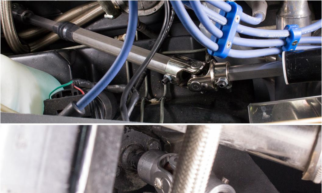
Place the U-joint for the steering box onto the 3/4" DD end of the collapsible shaft and connect the full assembly to the steering column U-joint. Adjust the collapsible shaft so that you are able to connect the U-joint to the steering box. Once everything is in place all bolts and setscrews must be tightened and locktite.
